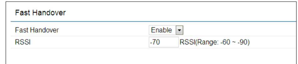
The screenshot shows the 'Fast Handover' settings. It includes a dropdown menu for 'Fast Handover' set to 'Enable' and a text input for 'RSSI' set to '-70'. A label 'RSSI(Range: -60 ~ -90)' is positioned to the right of the input field.
